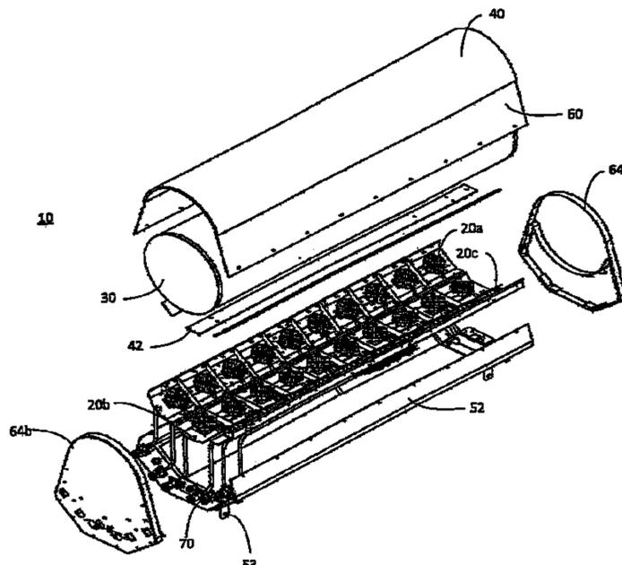
umns of radiating elements and the radio frequency lens. There may be more or fewer than two columns of radiating elements.
