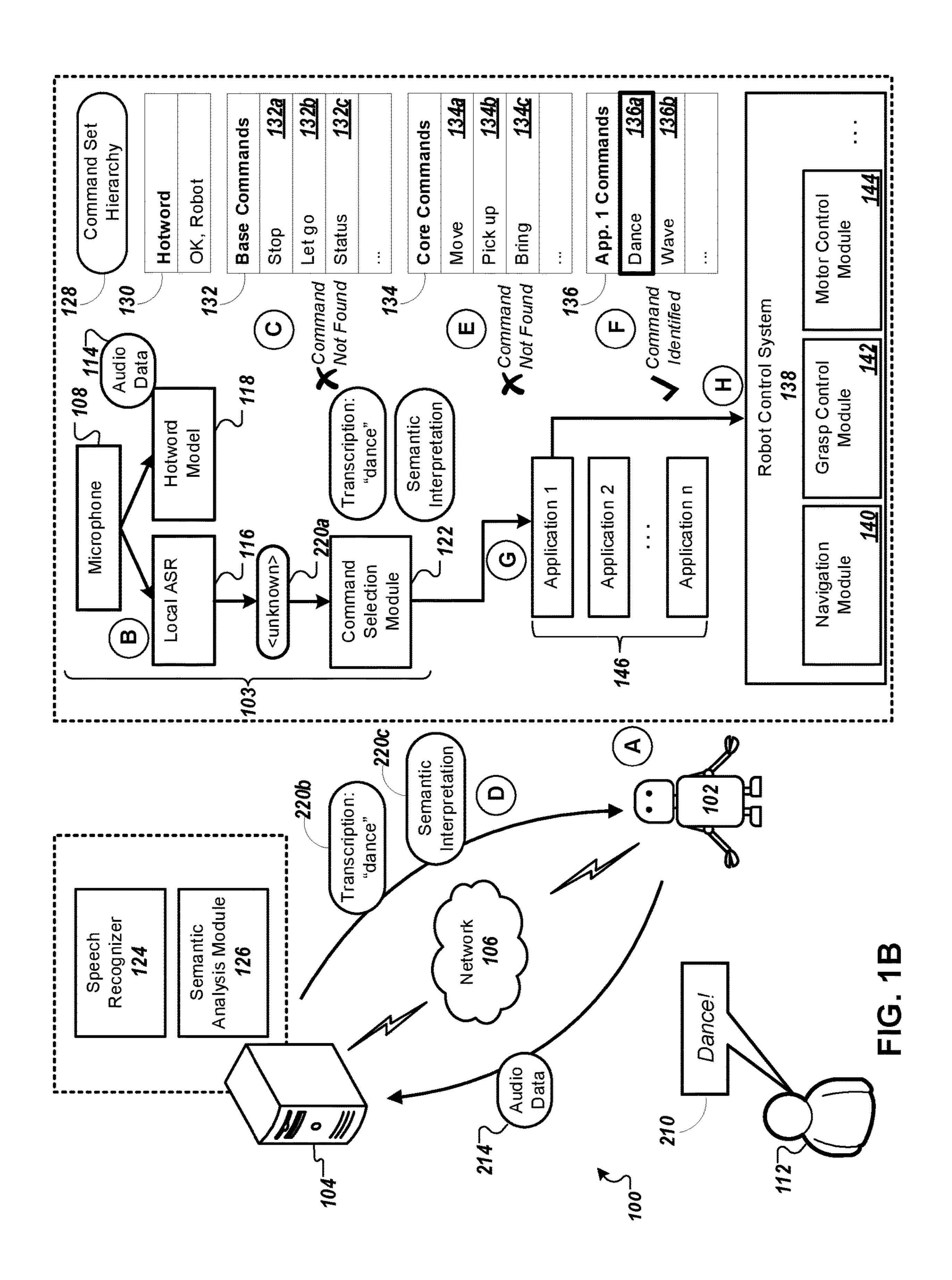
Operate, by the robot, an audio processing system to detect utterance of voice commands in a set of first commands that control behavior of the robot and in a set of second commands that control behavior of the robot
