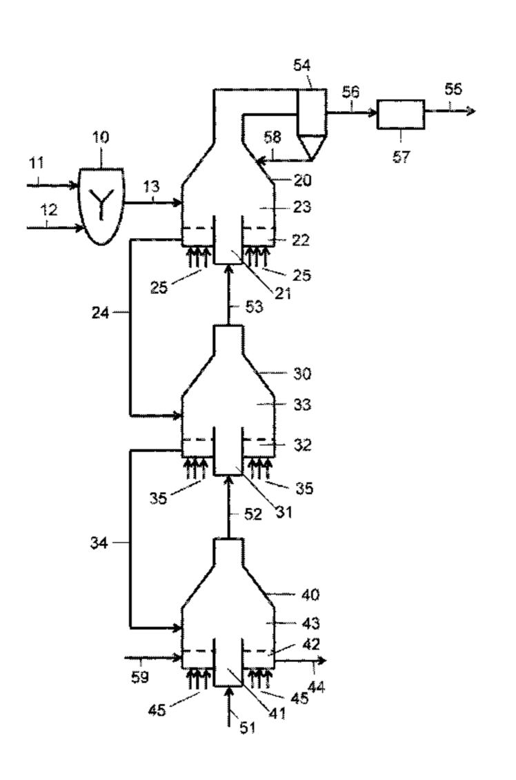
gas for a thermal treatment at temperatures between 200 and 1000° C. The at least one fluidized bed is developed such that it at least partly surrounds a gas supply tube for a gas or a gas mixture fed into the reactor and the gas or gas mixture is used as a heat transfer medium.
