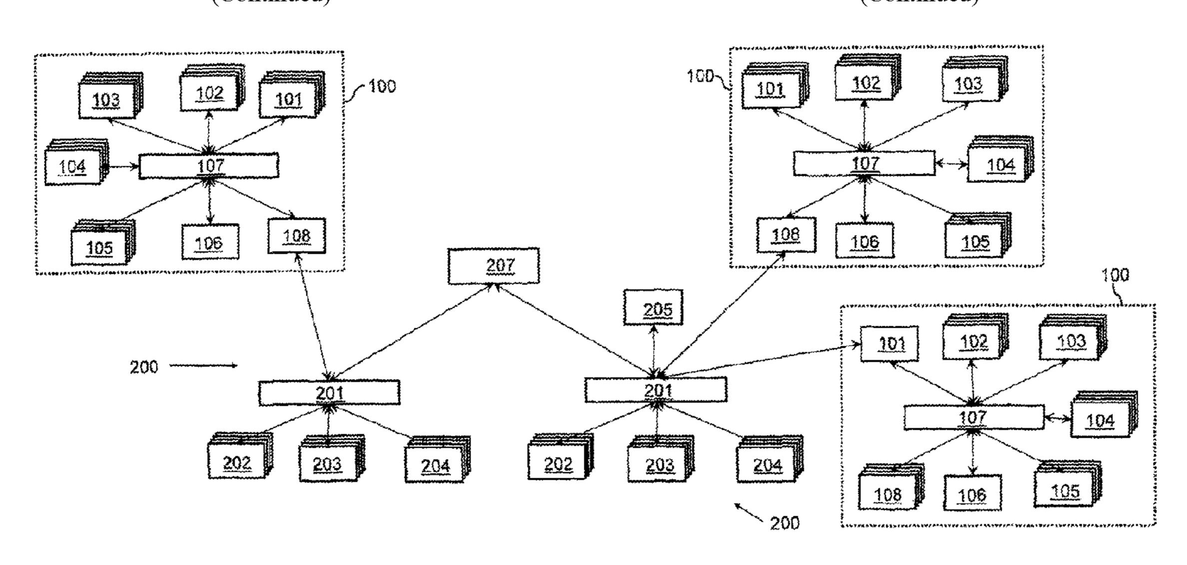
for carrying out data communication, wherein the client stations are coupled to each other via at least one external communication medium in order to carry out data communication. According to the invention, the client stations can communicate among each other. The invention furthermore relates to a computer system of this kind and a computer program for carrying out the method.
