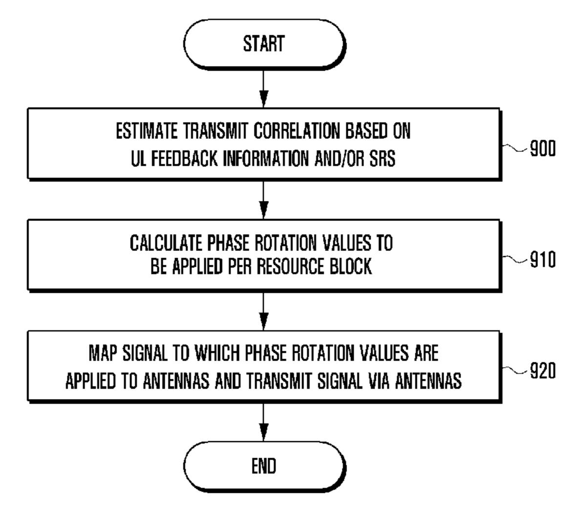
phase rotation value to be applied to a transmission signal on the basis of the estimated transmission correlation; applying a phase rotation in accordance with the phase rotation value to the transmission signal; and transmitting the transmission signal.
