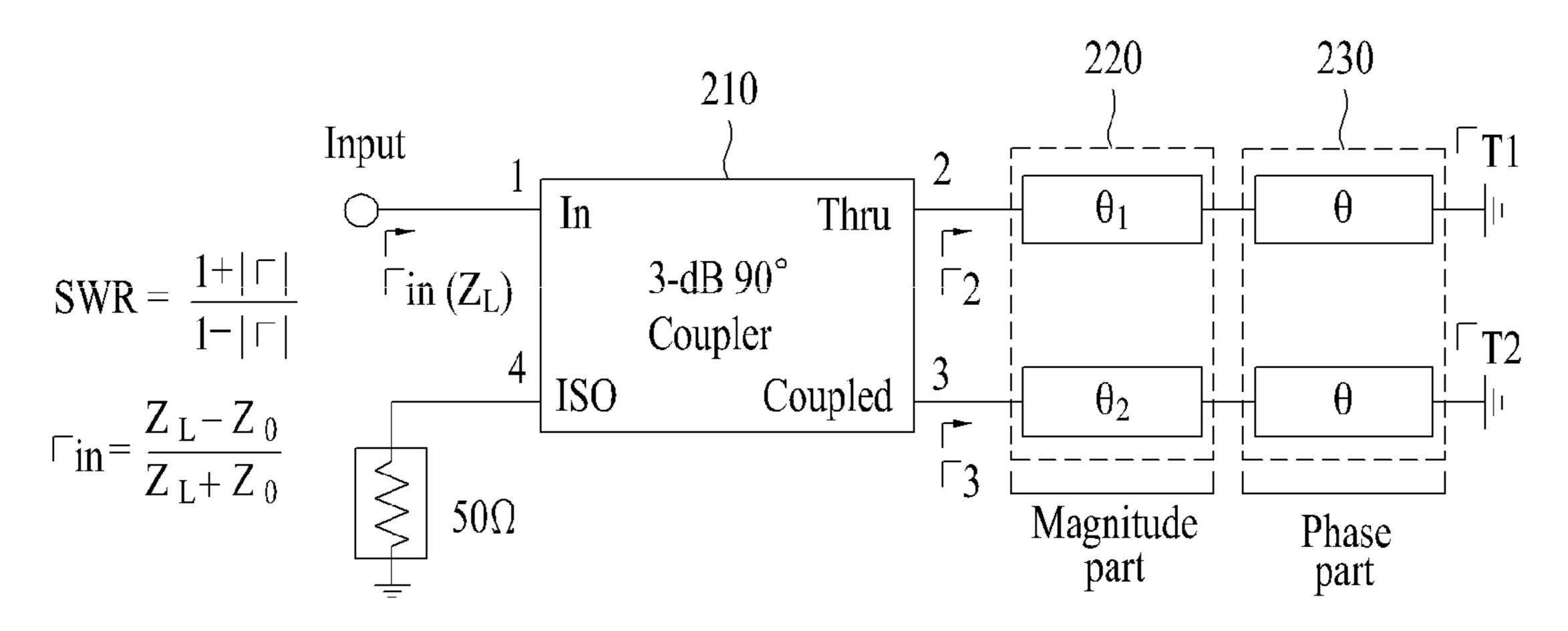
controlling a change in the phase of the impedance through an equal length change of the transmission lines.
