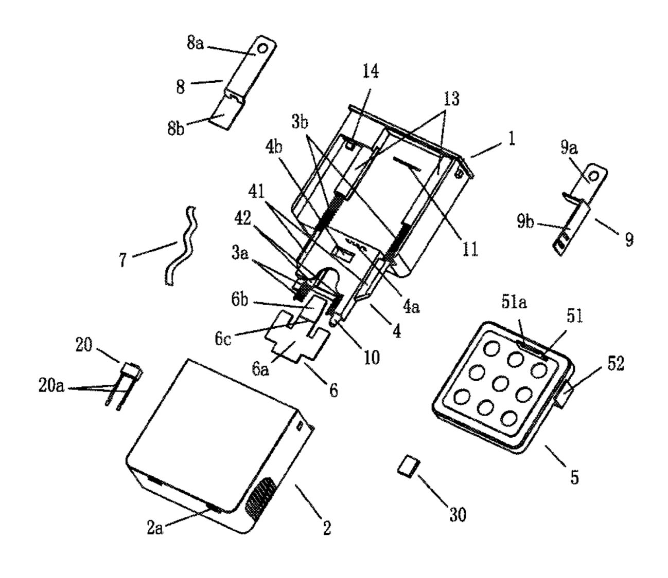
response of the thermosensitive element, meanwhile the response switch assembly is conceal by the arc-preventing assembly, thus preventing the arc generated when the switch is a catapulted and separated from forming a short-circuit and an overload, thus effectively avoiding fire and explosion hazards and further preventing secondary damage of electronic devices.
