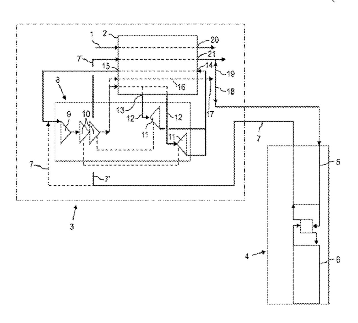
c): liquefying the nitrogen stream resulting from step a) in the main exchanger of the natural gas liquefaction unit in parallel with the liquefied natural gas in step b); wherein all the cold necessary for liquefying the stream of nitrogen and for liquefying the natural gas is supplied by the system for producing cold of the natural gas liquefaction unit.
