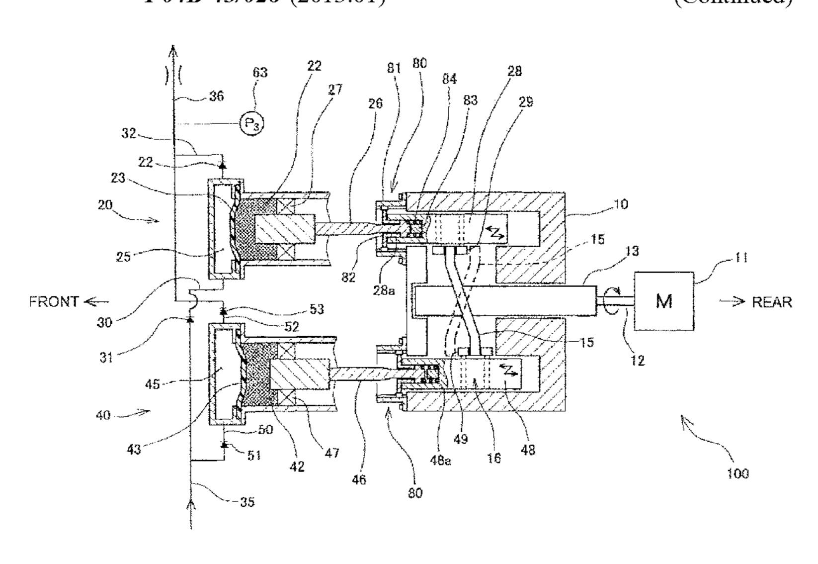
mechanism for adjusting the effective stroke length of the plunger in the preliminary compression step. Thus, generation of pulsation can be suppressed even when the set pressure changes.
