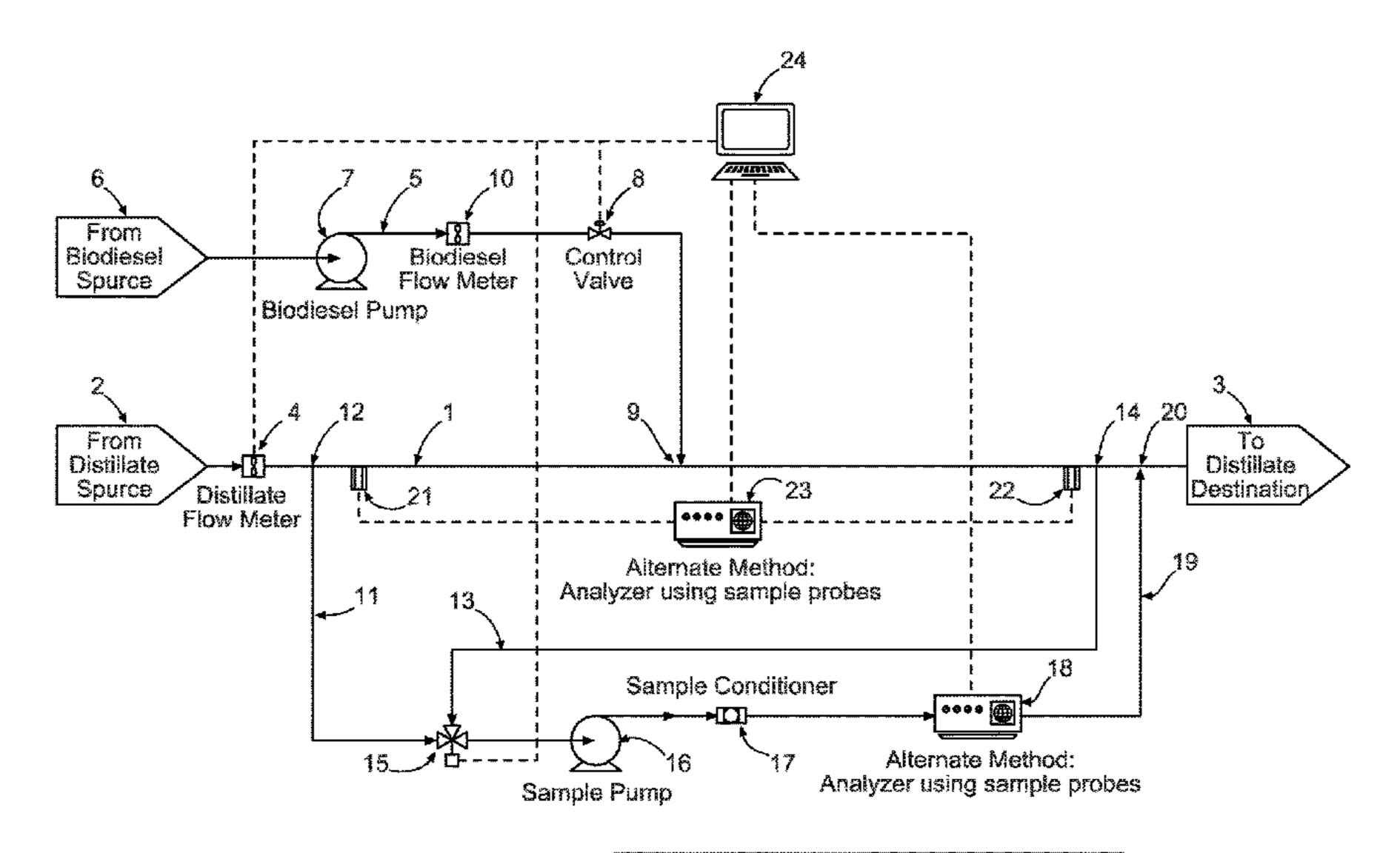
Controlled Blending of Biodiesel into Distillate Streams
