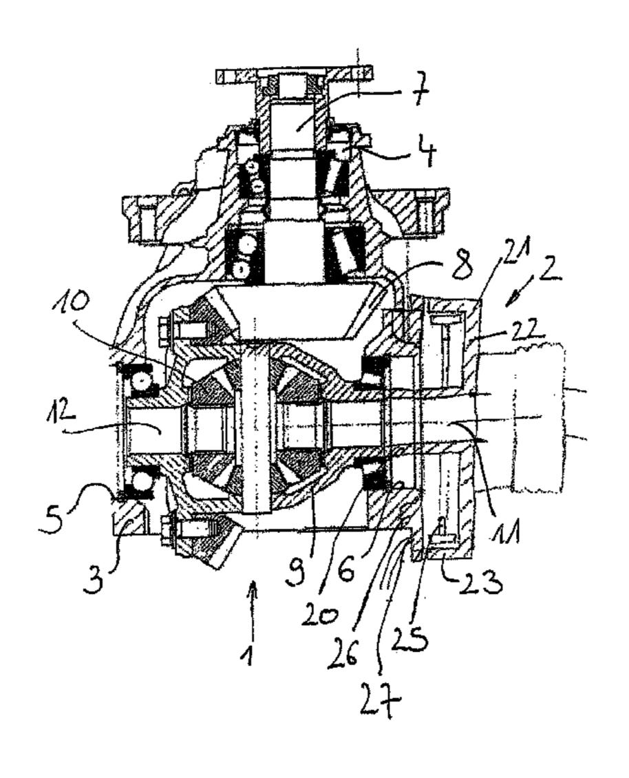
the frictional surfaces of which brake shoes can be placed against the cylindrical frictional surface of the passive element. The passive element can be a brake drum or a radial brake disk, the cylindrical edge of which serves as a frictional surface. The passive element is fastened to the differential cage and/or one of the shafts. The brake shoes are held in a pivotable manner on a carrier plate fastened to the outside of the differential housing.
