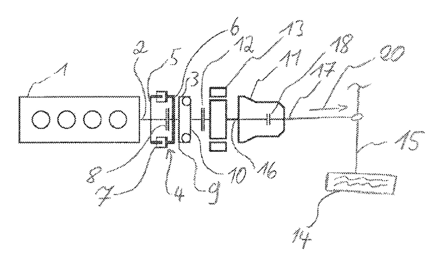
is arranged after the clutch device, relative to the torque transmission from the crankshaft in the direction of the drivable wheel. The clutch input side is connected to the crankshaft for conjoint rotation and the clutch output side is connected to the torsional vibration reduction device for conjoint rotation.
