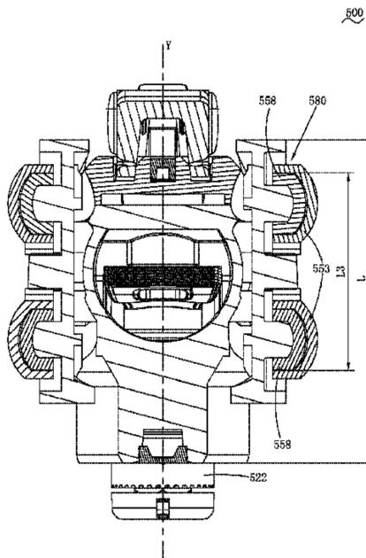
head housing. A sum of the lengths of the N vibration damping parts along the axial direction of the output shaft is larger than or equal to 0.2L and smaller than or equal to L. Therefore, a better vibration damping effect is achieved while working efficiency is not affected.
