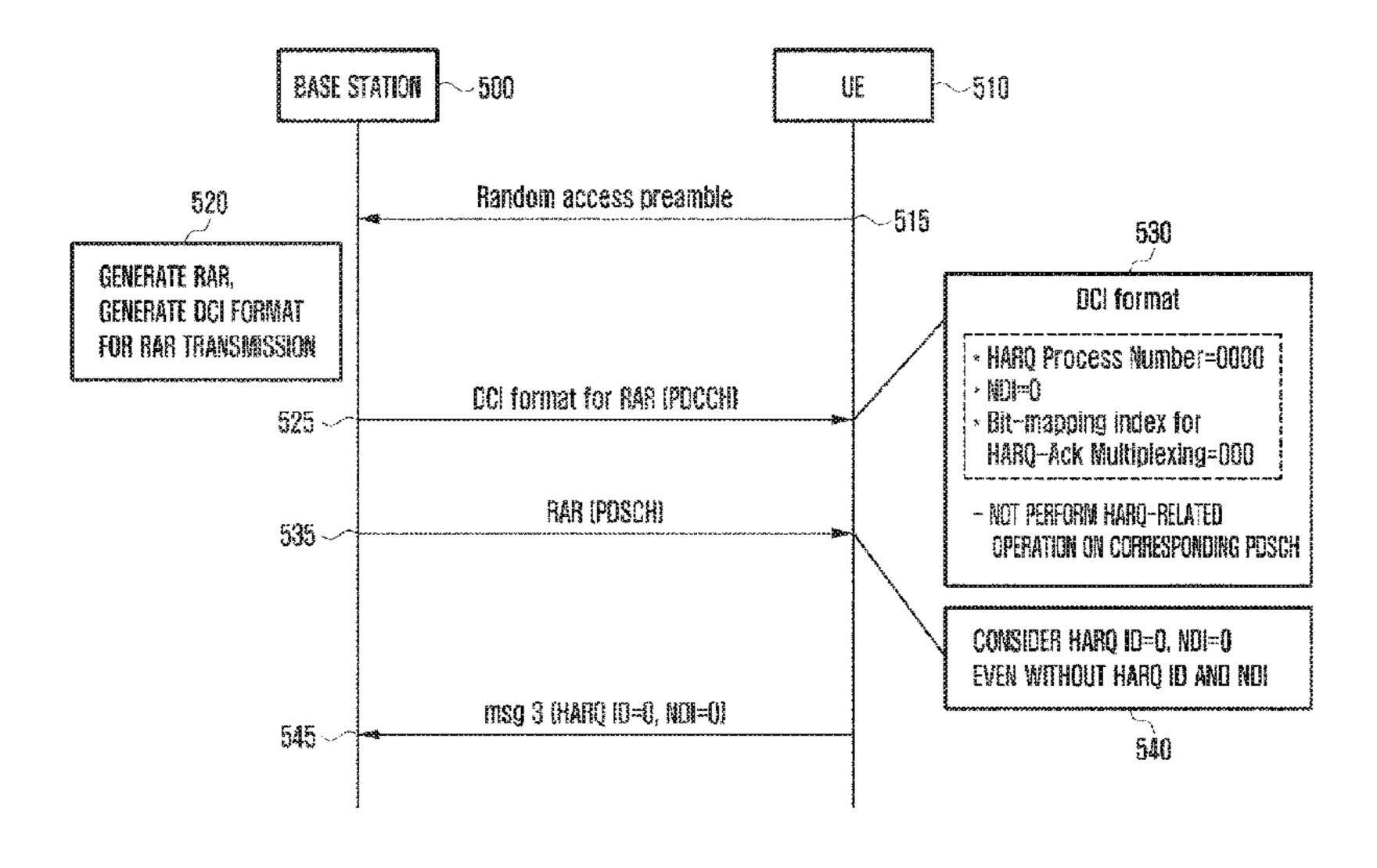
device for effectively transmitting or receiving control information for random access in a communication system. According to various embodiments of the present invention, information related to initial random access can be effectively transmitted and received.
