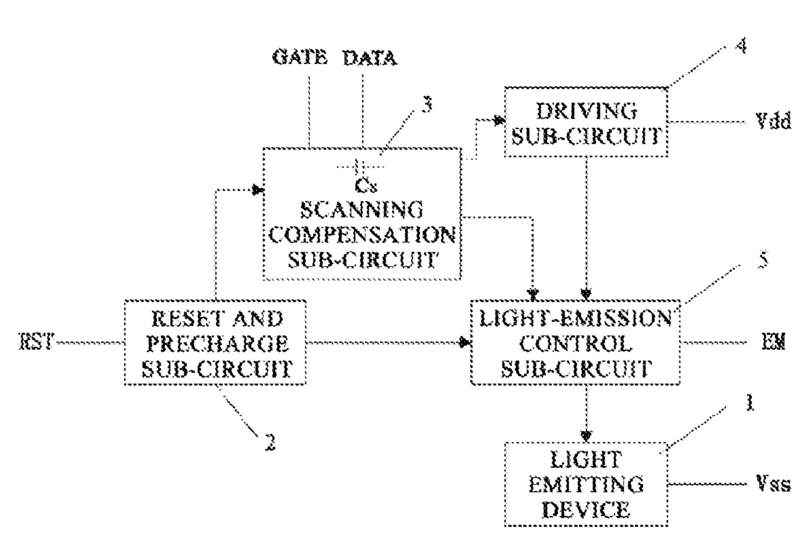
sion control sub-circuit, and is configured to reset the light-emission control sub-circuit according to a reset signal, and reset a second electrode of the storage capacitor of the scanning compensation sub-circuit according to a scanning signal; the scanning compensation sub-circuit is further coupled to the driving sub-circuit and the light-emission control sub-circuit, and is configured to charge the storage capacitor of the scanning compensation sub-circuit according to the scanning signal.
