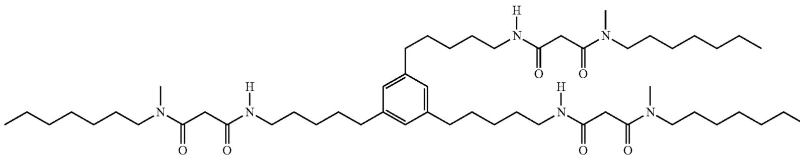
6. The illustrative magnesium sensing membrane of embodiment 1, wherein the ionophore is represented by the structure of Formula IV:
