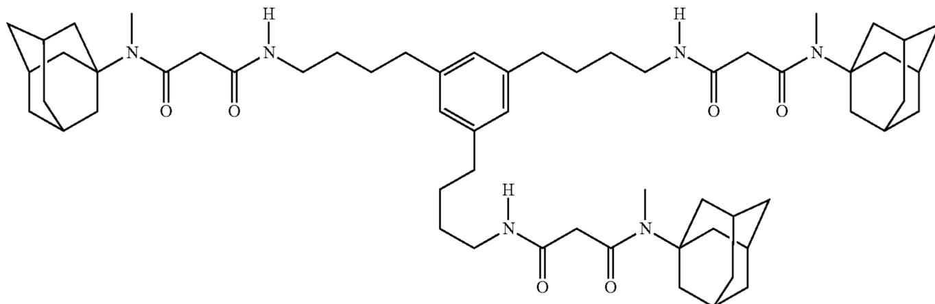
5. The illustrative magnesium sensing membrane of embodiment 1, wherein the ionophore is represented by the structure of Formula III:
