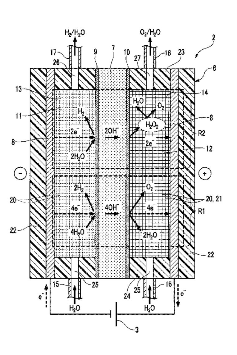
exchange membrane; a cathode feeder that is arranged within the cathode chamber and feeds power to the cathode; an anode feeder that is arranged within the anode chamber and feeds power to the anode; and an active oxygen reduction material that is arranged within the anode chamber and reduces active oxygen generated within the anode chamber.
