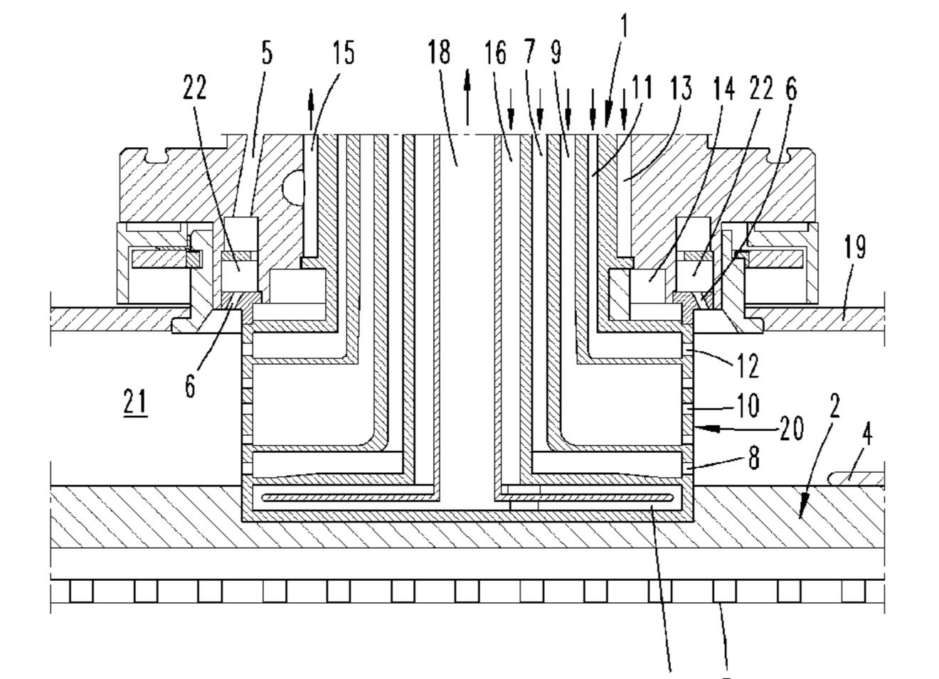
the susceptor is heated to at least 700° C. At the same time, the passivation layer is formed by chemically reacting a metal-organic compound with the metal atoms of the metal surface. The cleaning gas inlet openings are arranged such that the cleaning gas comes into contact with the metal surface that has the passivation layer.
