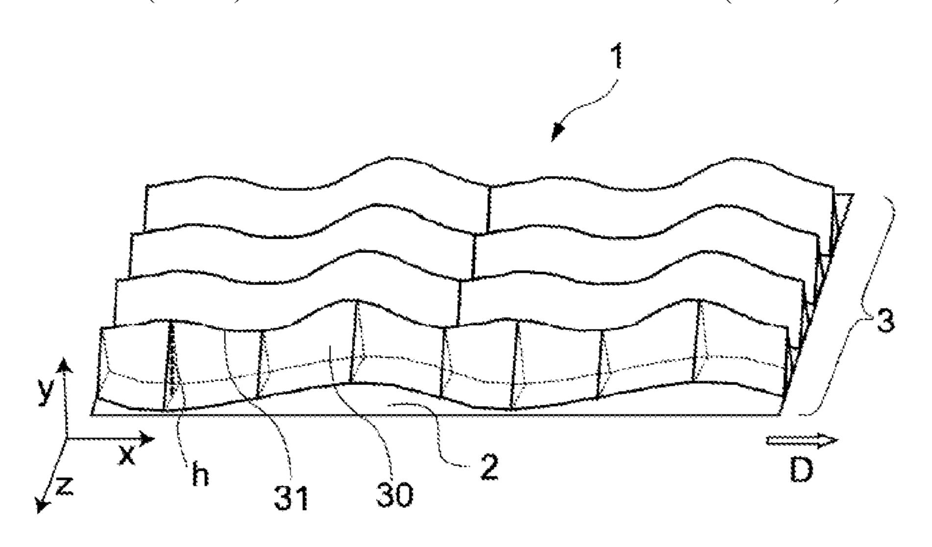
line, and a height thereof changes cyclically with respect to a fluid flow direction. With such a configuration, drag, which is a sum of turbulent friction drag and pressure drag, can be further reduced.
