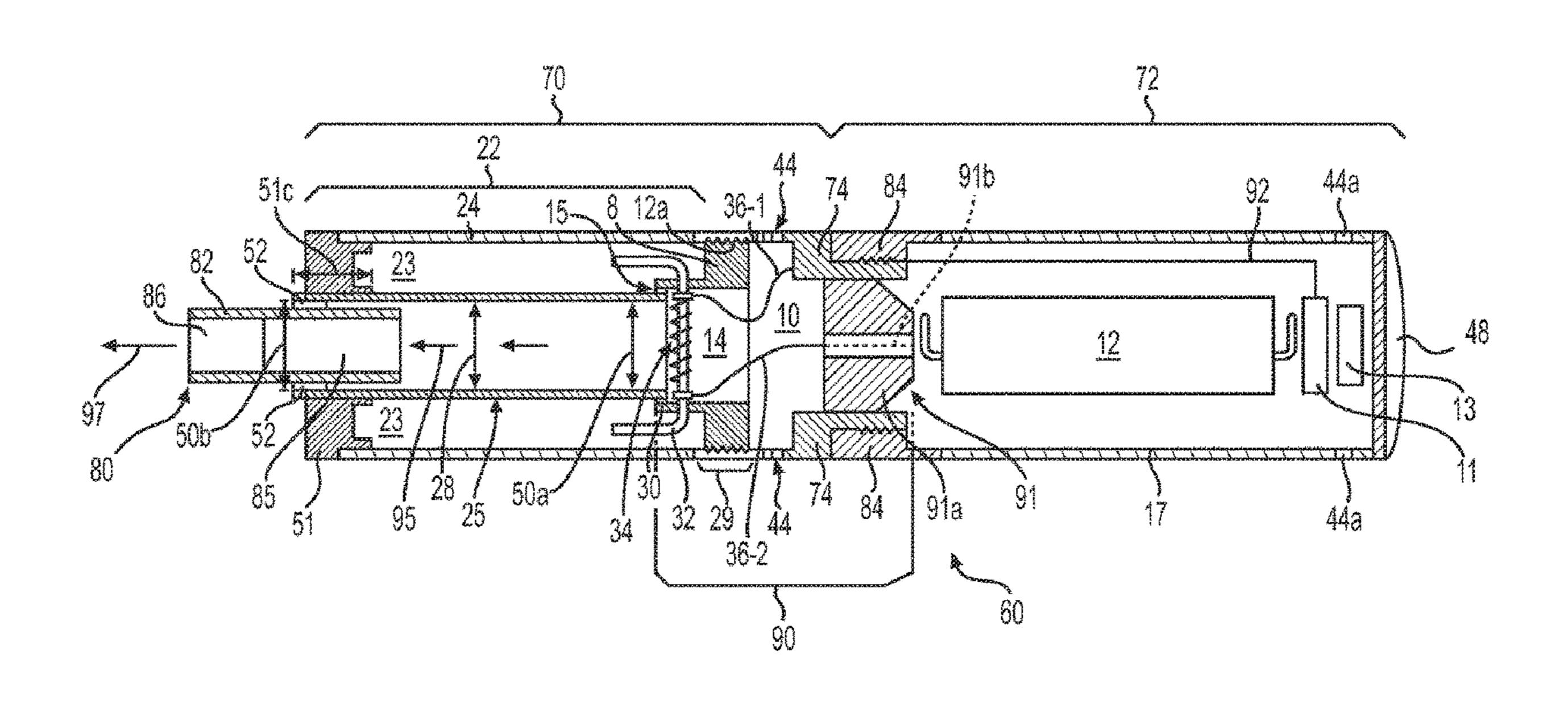
insert and the vaporizer assembly may be at opposing ends of the channel. The flavor insert may be a detachable insert configured to be inserted into the tank element. The flavor element may be a tobacco element. The tobacco element may be at least a portion of a cigarette.
