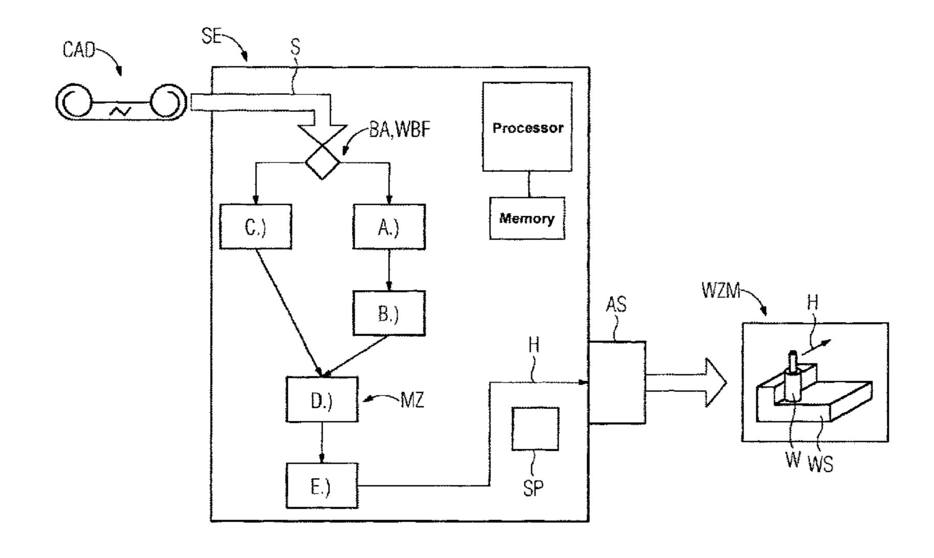
travel profile such that the travel profile can be optimized via the selection of wavelet base functions, based on a processing mode, e.g. rough milling, fine milling, laser cutting.
