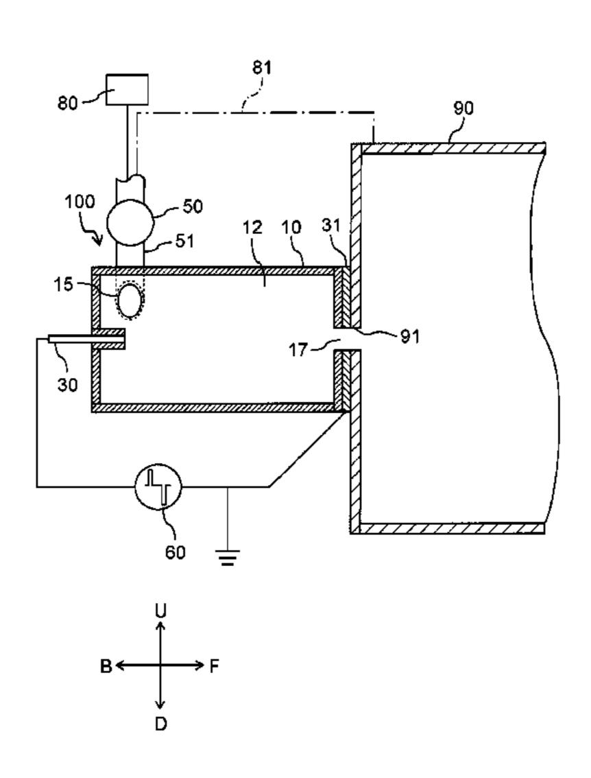
first electrode and the second electrode so as to generate plasma in the gas phase. A reformed liquid is produced in a manner that the plasma is generated in the gas phase so as to form a reformed component, and the formed reformed component is dissolved and dispersed in the liquid.
