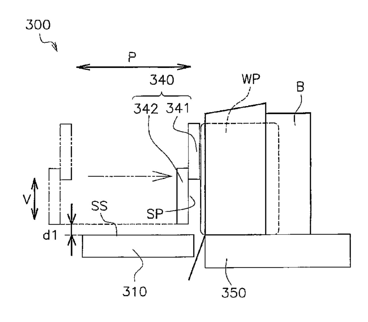
cate horizontally above the placement surface so that the push-in plate moves toward the box or moves away from the box. The lifting/lowering mechanism moves the push-in plate so as to change a separation distance in the height direction between a lower edge of the pressing surface and the placement surface.
