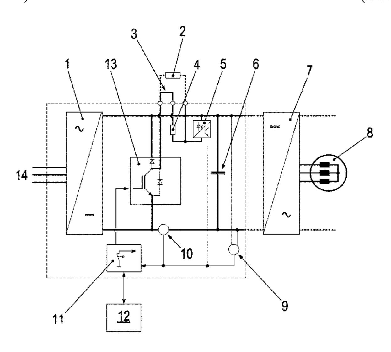
its set value toward the output signal of the device. The controller in particular has a linear controller element whose set value is forwarded to a difference generator for determining the difference between the set value and the value of the electric power, the set value being supplied, directly or via a limiter, to a parameterizable filter.
