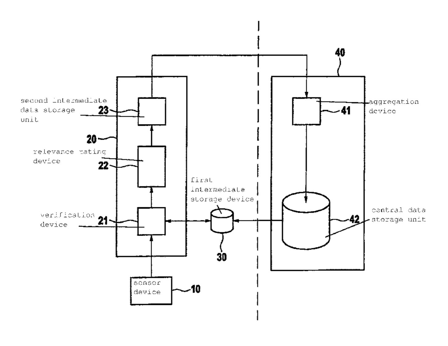
the acquired surrounding-area data to known surroundingarea data of a data storage unit of a server device; and uploading the acquired surrounding-area data to the server device (40) as a function of the evaluation.
