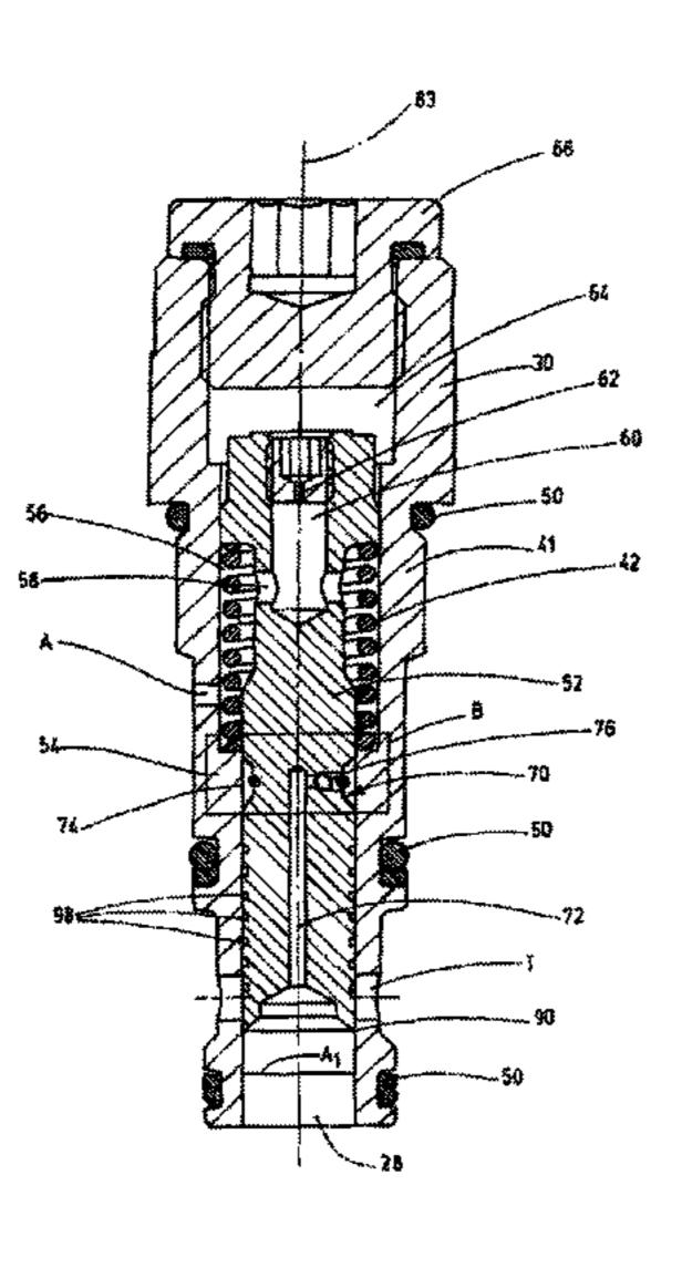
a pressure-compensated manner due to the force of the energy accumulator (42).
