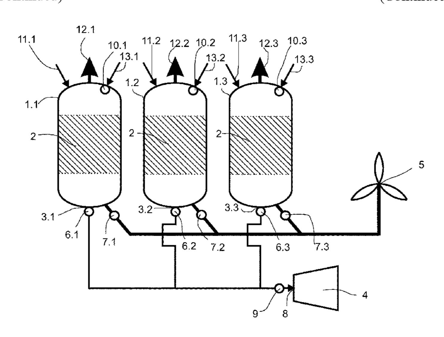
fied combustion for automatically increasing pressure of the combustion gases and using them in a combustion engine for performing mechanical work, the above-stated problem is solved in that an oxygen storage material is present in the combustion space so that a self-compressing combustion process is made possible by storing the oxygen in the oxygen storage material in the combustion space.
