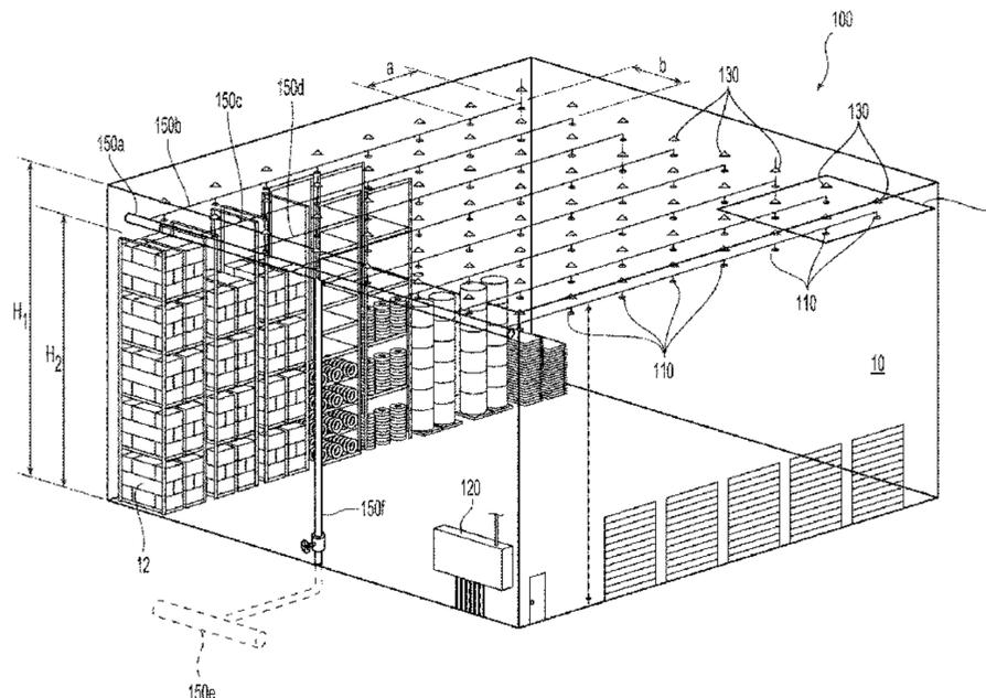
protected may include exposed expanded plastics. The fluid distribution devices include a frame body having an inlet, an outlet, a sealing assembly, and an electronically operated releasing mechanism supporting the sealing assembly in the outlet.
