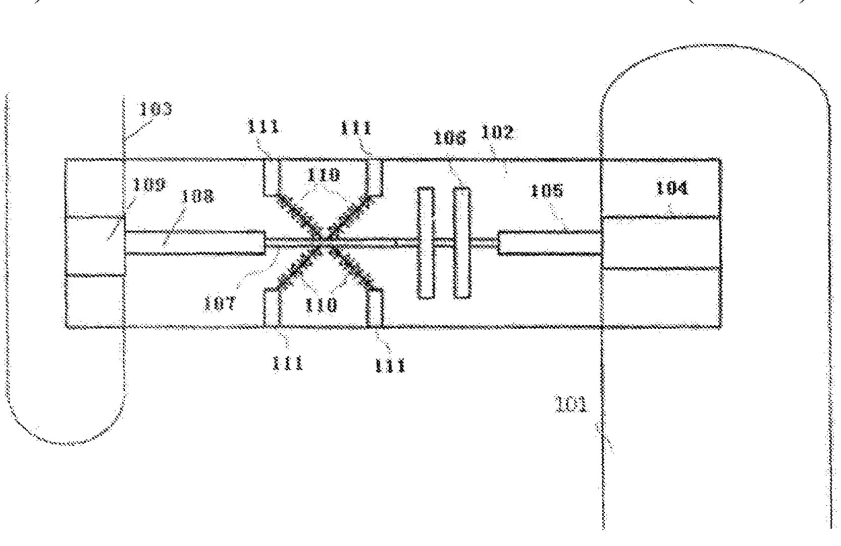
sion microstrip, a low pass filter, a RF matching microstrip and a second transmission microstrip, where anodes of four GaAs-based terahertz frequency multiplier diode groups are connected to the RF matching microstrip, and a cathode at the outermost position of each of the GaAs-based terahertz frequency multiplier diode groups is connected to a grounding quartz strip.
