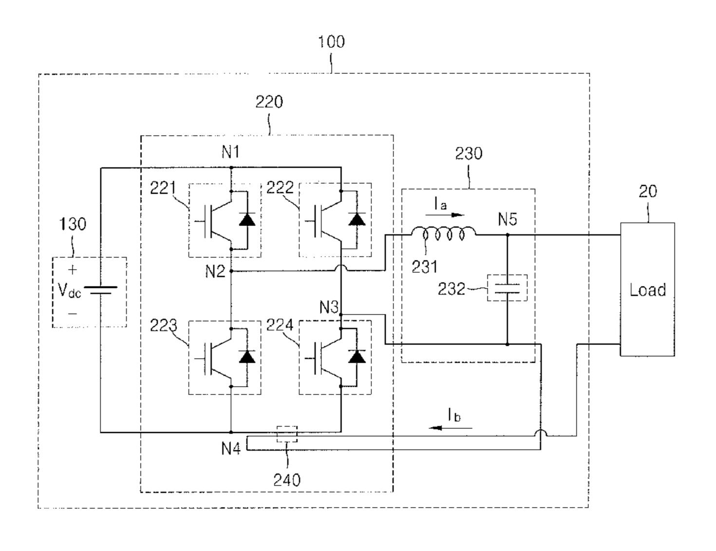
output current is output to a load connected between the third and fifth nodes.
