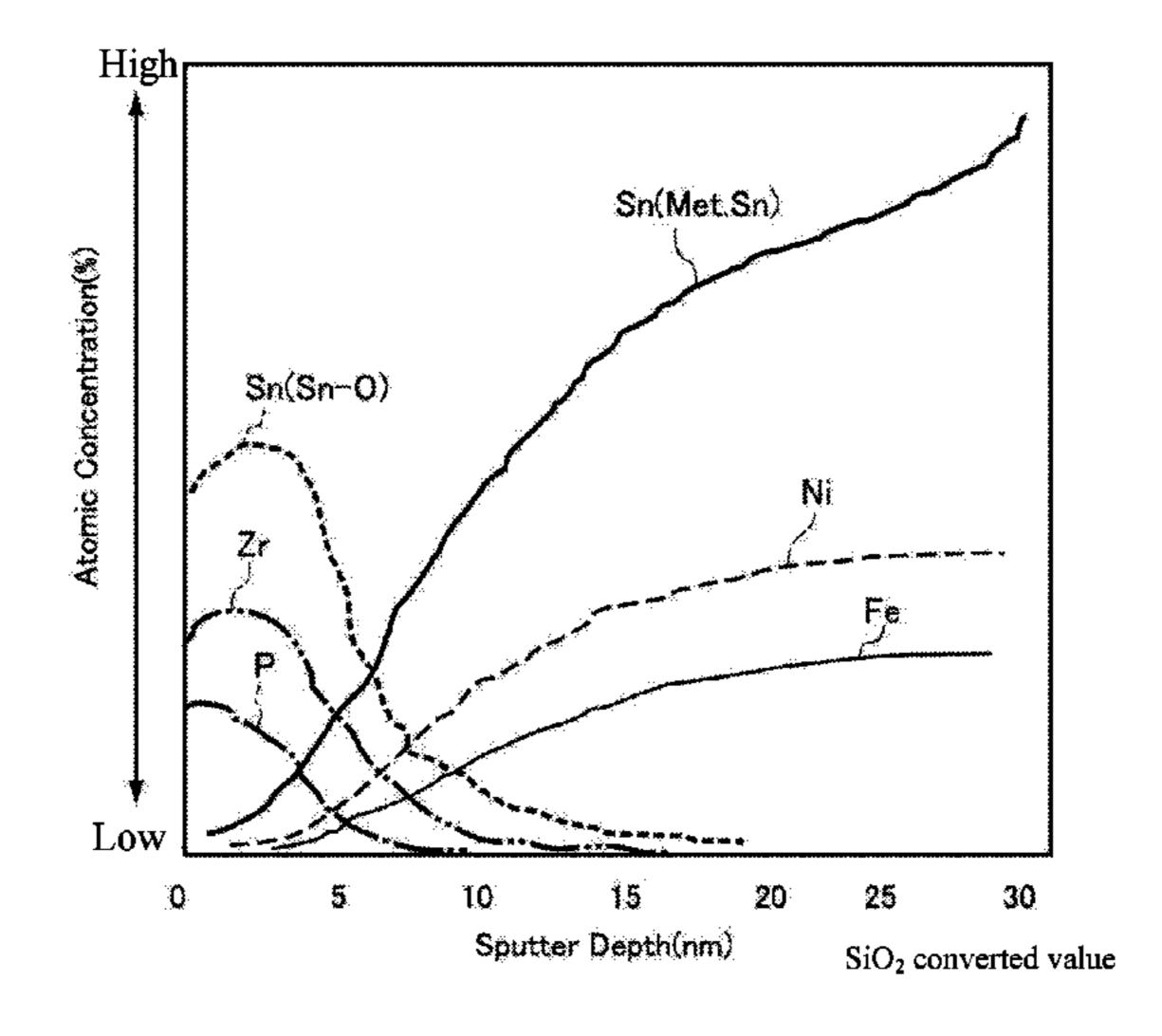
amount of Sn, a content of the zirconium oxide in the coating layer is from 0.2 mg/m<sup>2</sup> to 50 mg/m<sup>2</sup> in terms of metal Zr amount, and a peak position of binding energy of Sn3d<sub>5/2</sub> according to X-ray photoelectron spectroscopy of the tin oxide in the coating layer is 1.6 eV or higher than a peak position of binding energy of the metal Sn.
