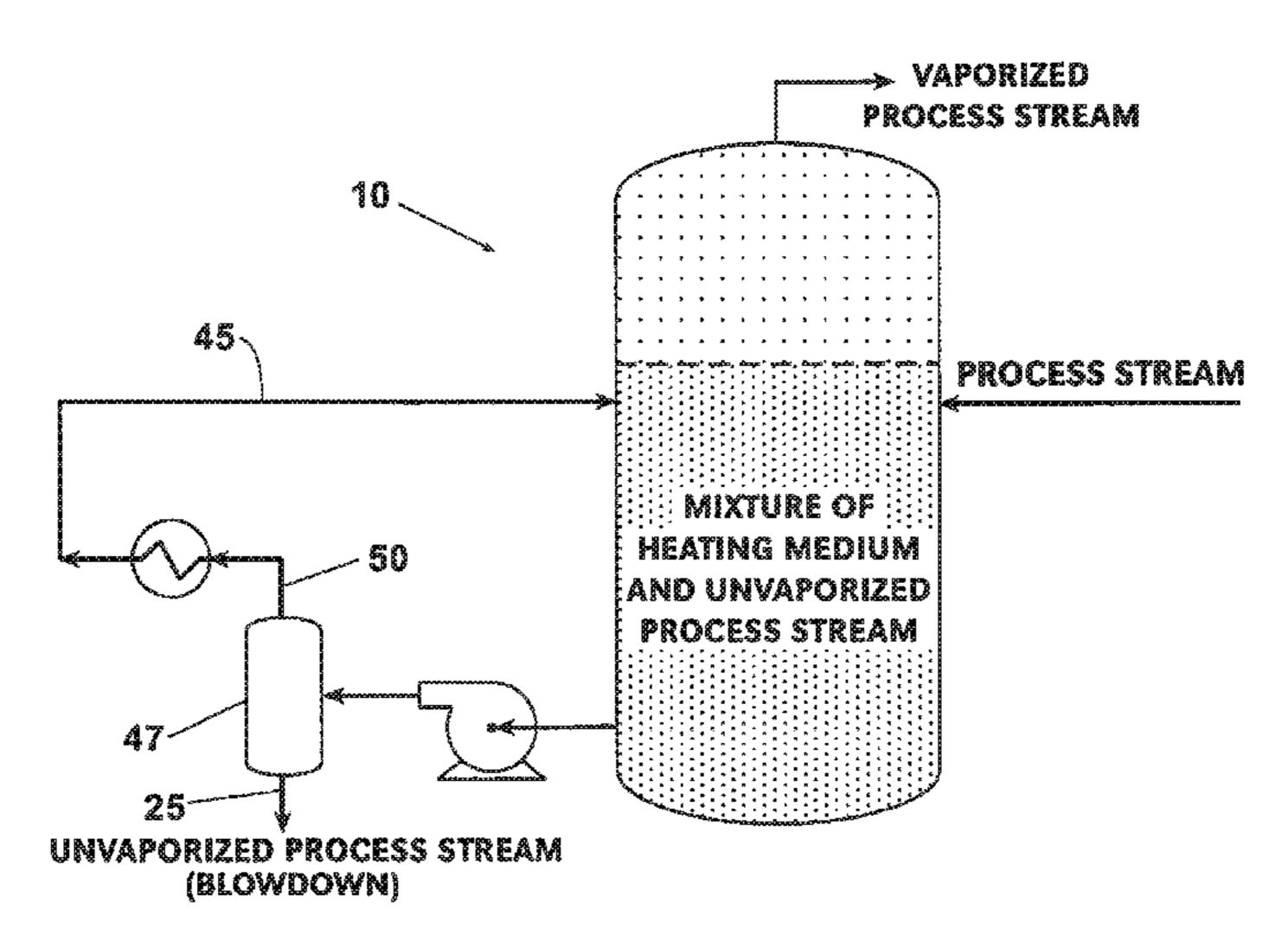
pump-around loop. The vaporized process stream can be further condensed. Any heat recovered can be used to pre-heat the process stream or in the pump-around loop's heater in case of mechanical vapor recovery.
