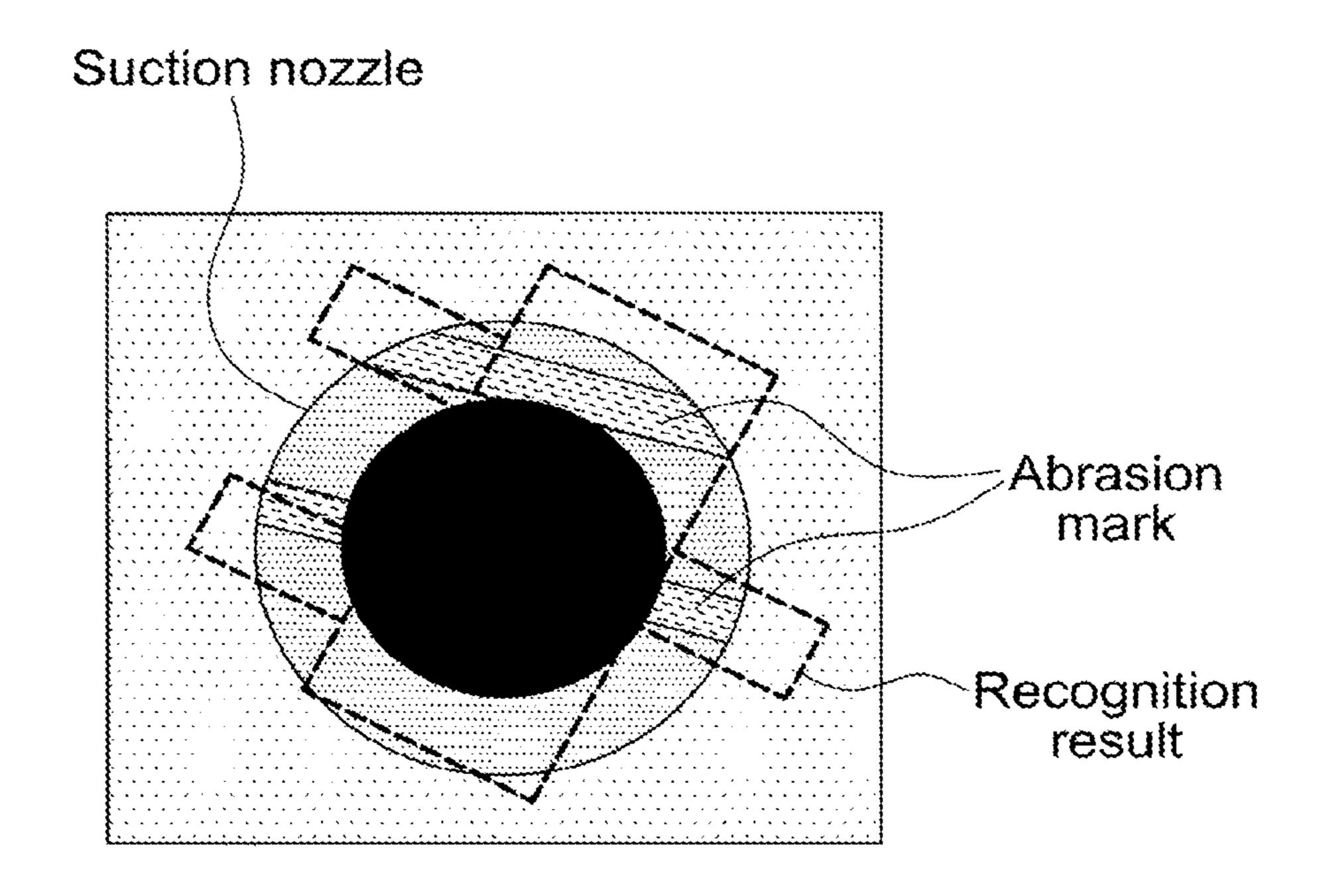
Misrecognition due to suction nozzle abrasion mark
