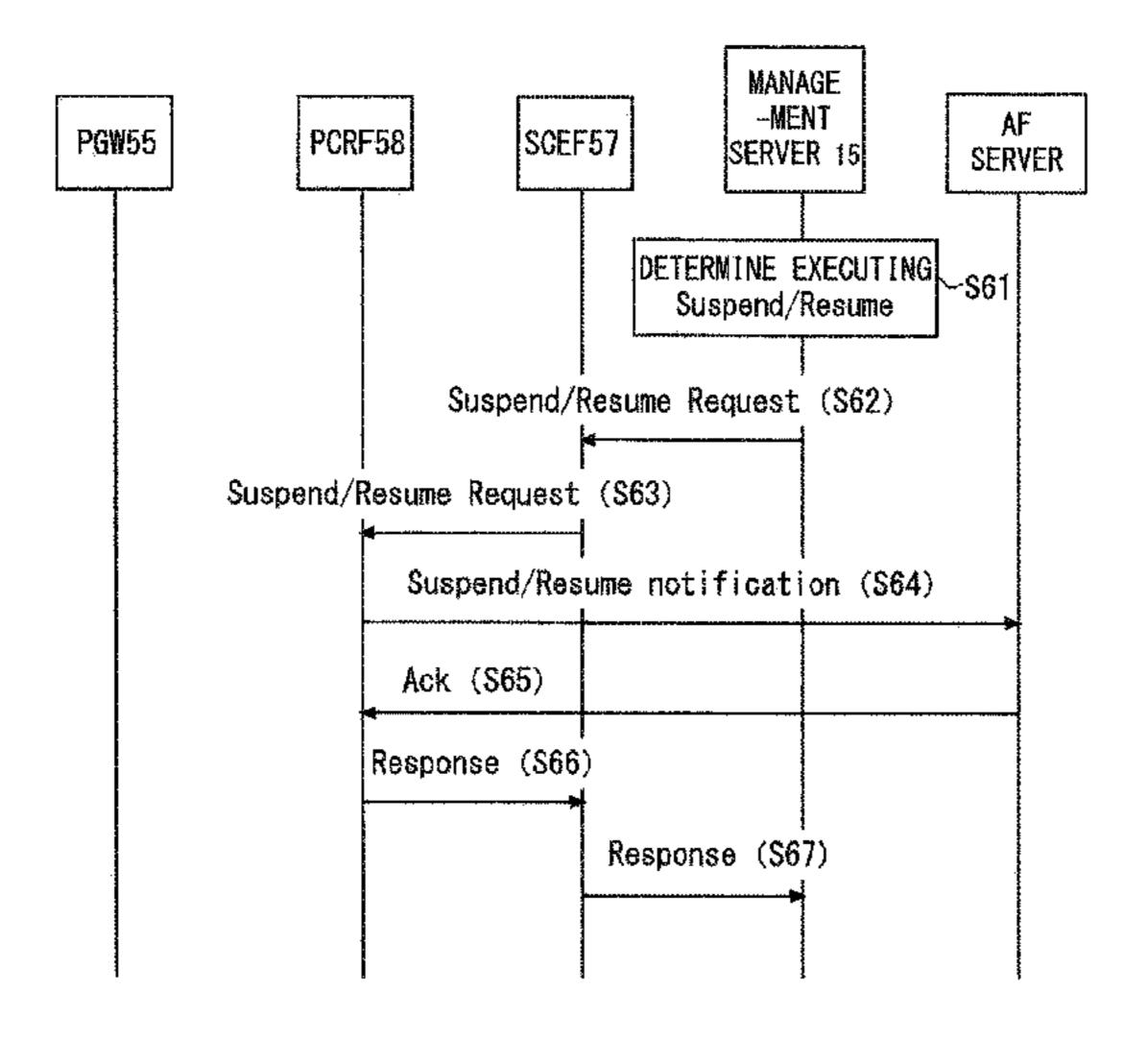
the communication related to the communication terminal, stopping transmission of data to the communication terminal and stopping transmission of data transmitted from the communication terminal to another communication apparatus.
