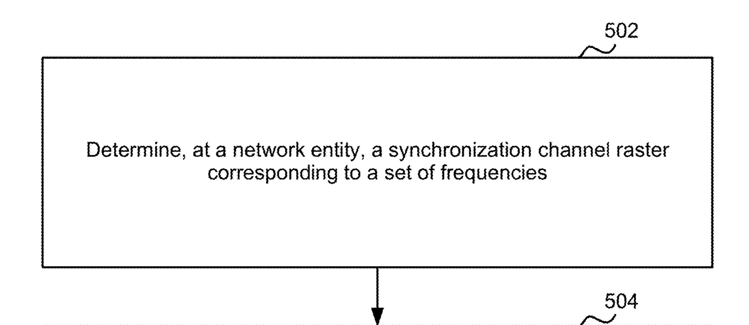
Transmit, from the network entity, one or more synchronization signals and a physical broadcast channel (PBCH) in a frequency of the set of frequencies of the synchronization channel raster closest to a center frequency of a bandwidth
