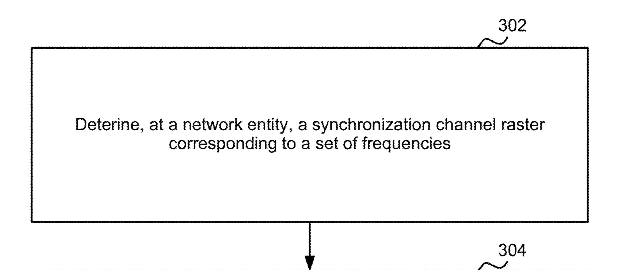
Transmit, from the network entity, one or more synchronization signals and a physical broadcast channel (PBCH) in any frequency of the set of frequencies of the synchronization channel raster to at least one user equipments (UE)
