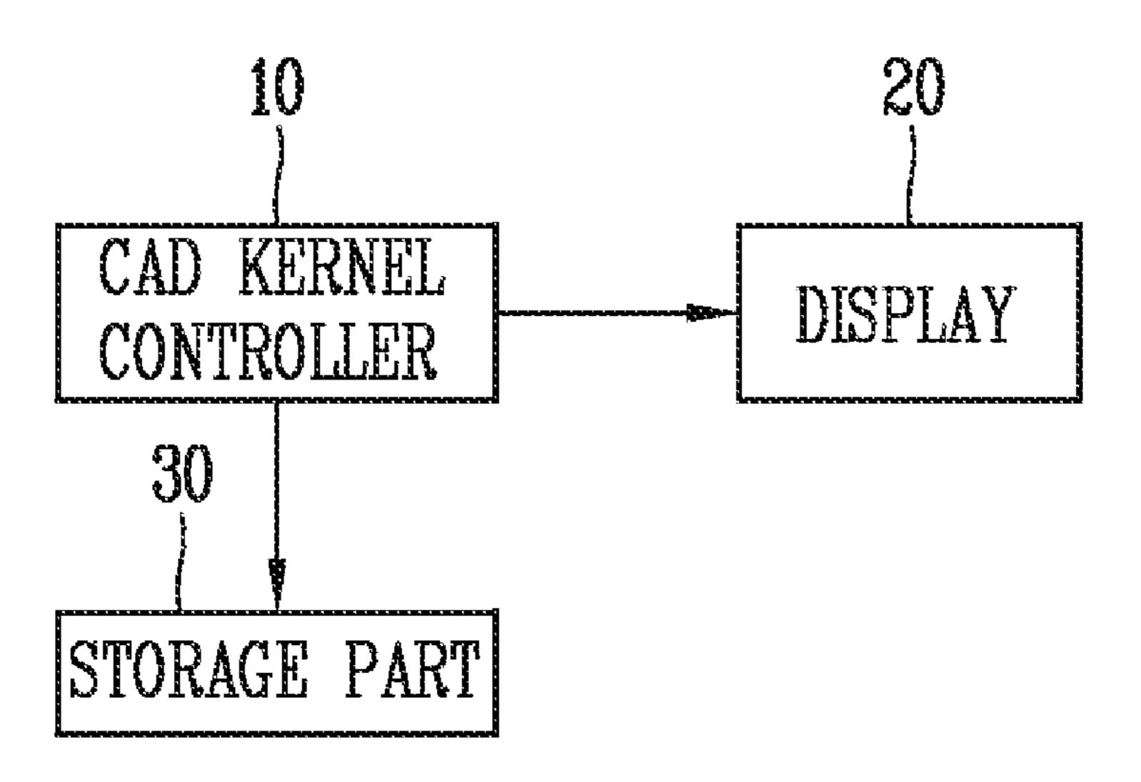
cutting target in a nuclear facility by using a design program, displays the cut shape on the display unit, and predicts the amount of secondary waste generated in the process of cutting the cutting target.
