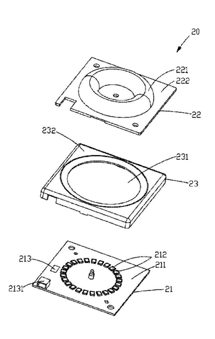
part is bonded to the substrate and is configured to fix the optical element above the at least two luminescent units.
