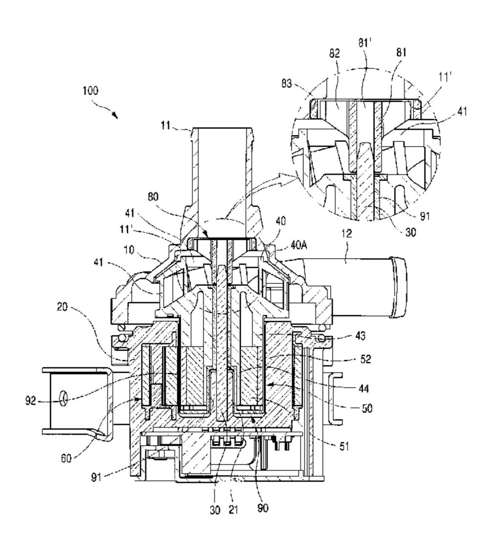
of the shaft fixing support and around the shaft, and a second synthetic resin mold around an outer side of the rotor.
