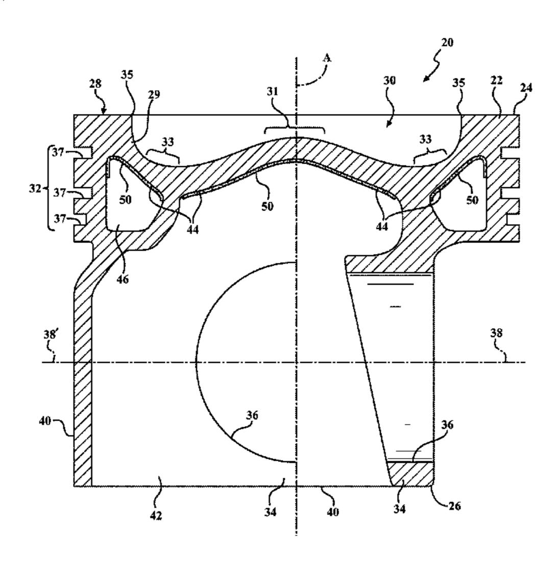
wherein an insulating coating is applied to at least one of the portions of the undercrown surface.
