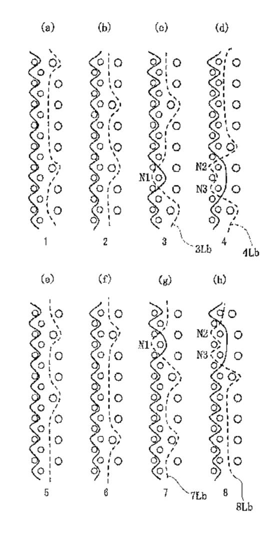
formed and includes at least two or more knuckles which are formed by passing over another upper surface side warp or another upper surface side weft located adjacent to said upper surface side warps or said upper surface side wefts.
