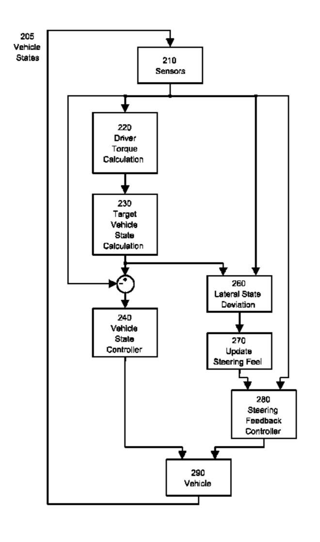
results in a yaw and/or lateral vehicle state error, this error is transformed to a change in the steering-wheel torque to steering-wheel angle relation describing steering feel. This new steering feel relation is used as an input signal for controlling the feedback torque actuator in order for the driver to get feedback of the yaw and/or lateral vehicle state error.
