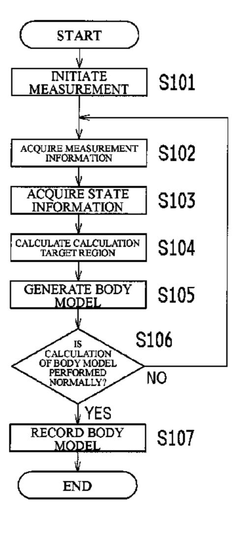
lation target region by approximately determining a circle or sphere having the length from the rotation center to the calculation target region as a radius using a mathematical method such as a least-squares method on the basis of the measured information acquired over time. Then, the calculation device records the calculated body model in a body model recording unit.
