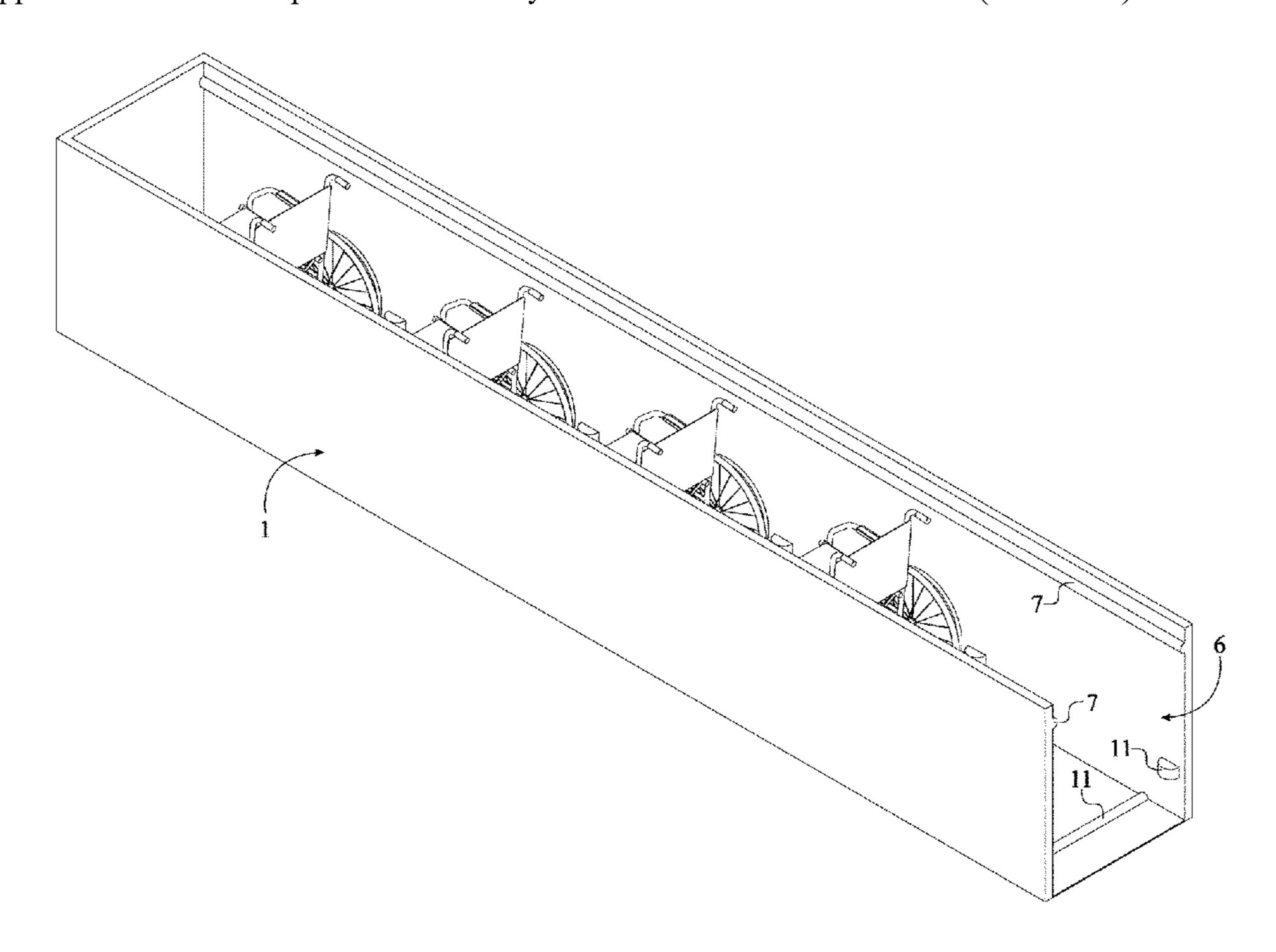
wheelchairs. The entrance is delineated by the first wall and the second wall and provides an opening to enter the floor mounted enclosure. The at least one guard rail internally connected to the floor mounted enclosure to eliminate damages from the wheelchairs. The wheelchair stopper is integrated into the enclosure to secure the wheelchairs within.
