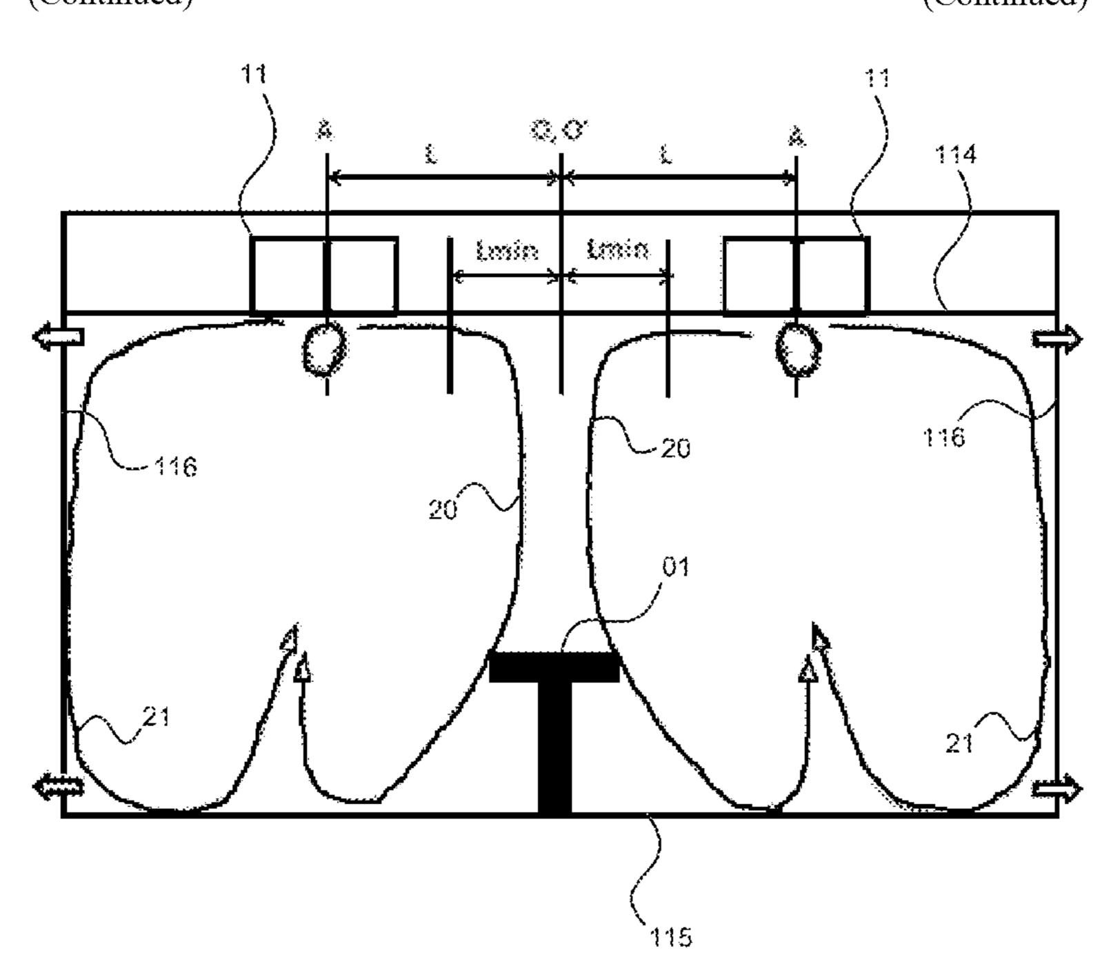
adjusted so that the substantial center of the critical area is flushed by the first flow and penetration of the second flow into the substantial center of the critical area is generally prevented. In other embodiments, a HVAC system and method are discussed along with the features of the device.
