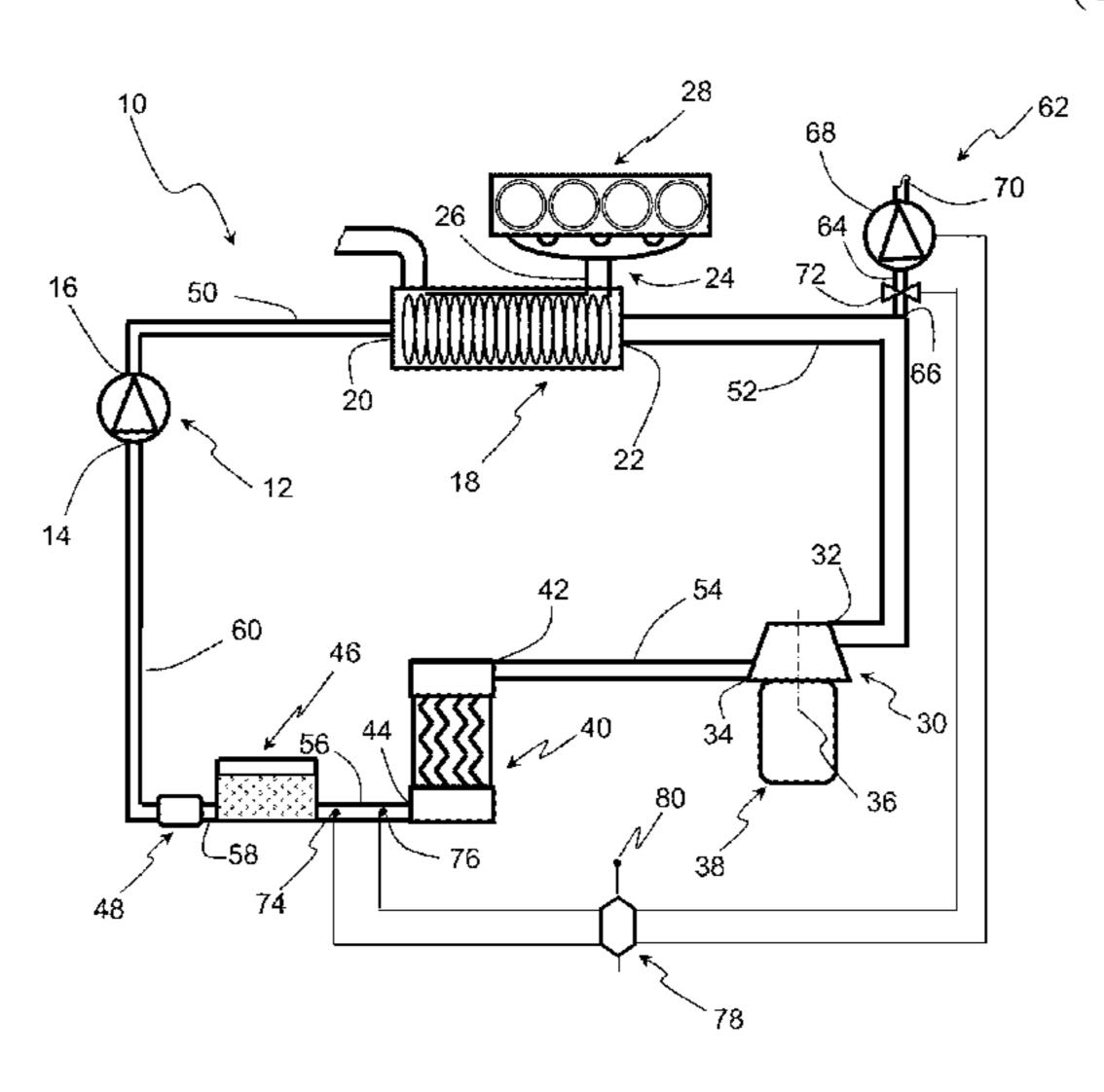
point of the loop when this loop is at rest, and, as soon as the measured pressure (Préelle) exceeds a threshold value (Pliquide saturé) for a given ambient temperature (T), activate equipment for extracting the gaseous fluid in order to discharge it from the loop.
