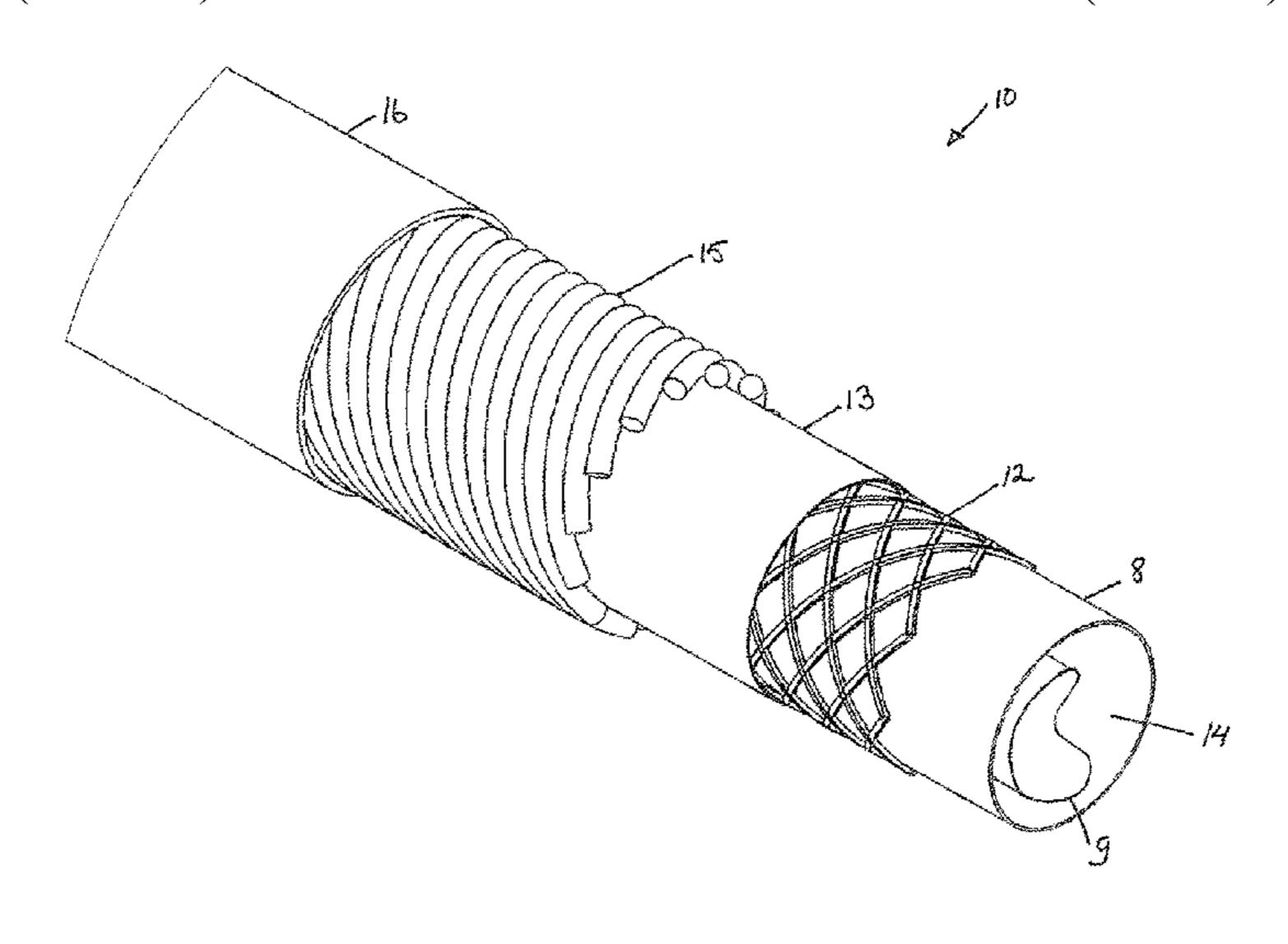
one of the plurality of electrical conductors through the outer layer. The braid underlies the at least one electrode but is insulated from the at least one electrode by the intermediate non-conductive layer.
