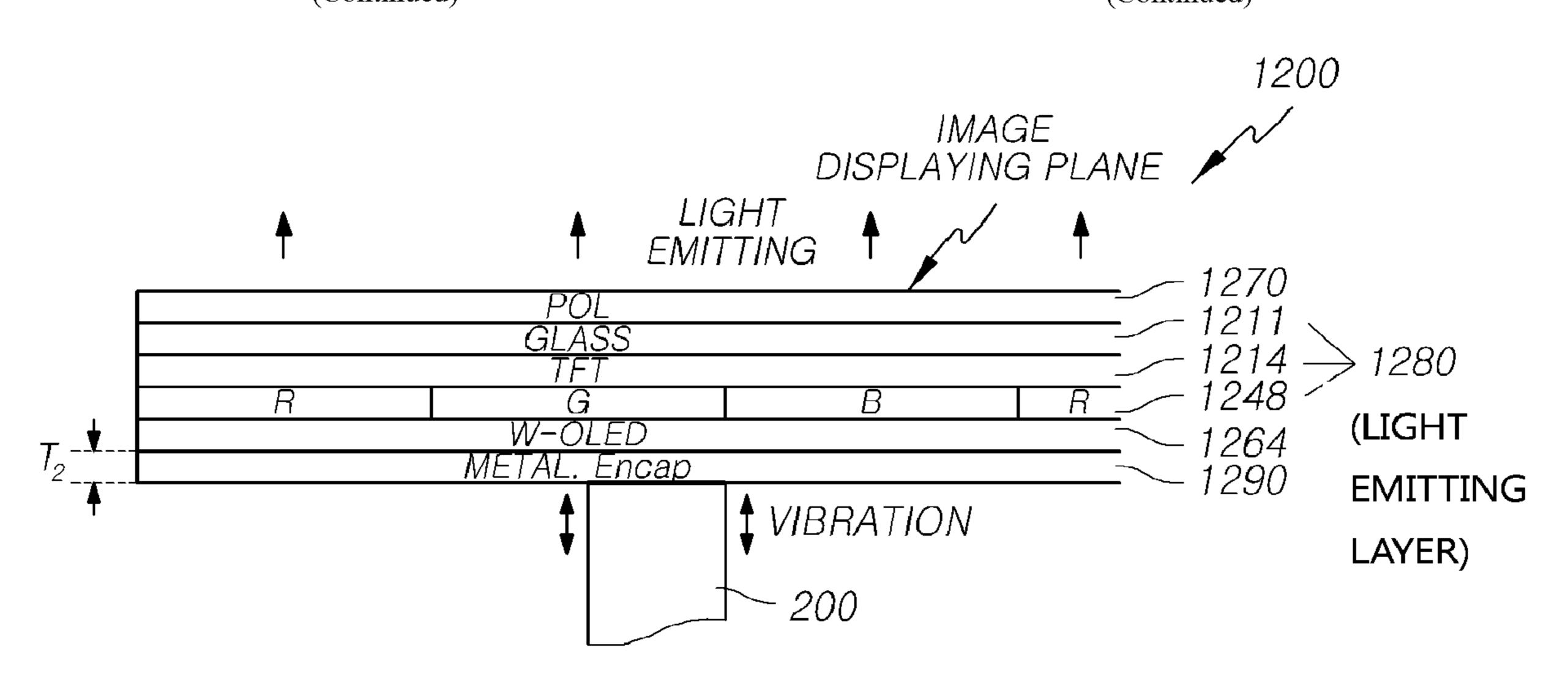
can prevent generation of a weighted color mixing phenomenon in a wide viewing angle at the time of panel vibration and reduce the thickness or weight of the panel to thereby enhance the sound generation characteristic.
