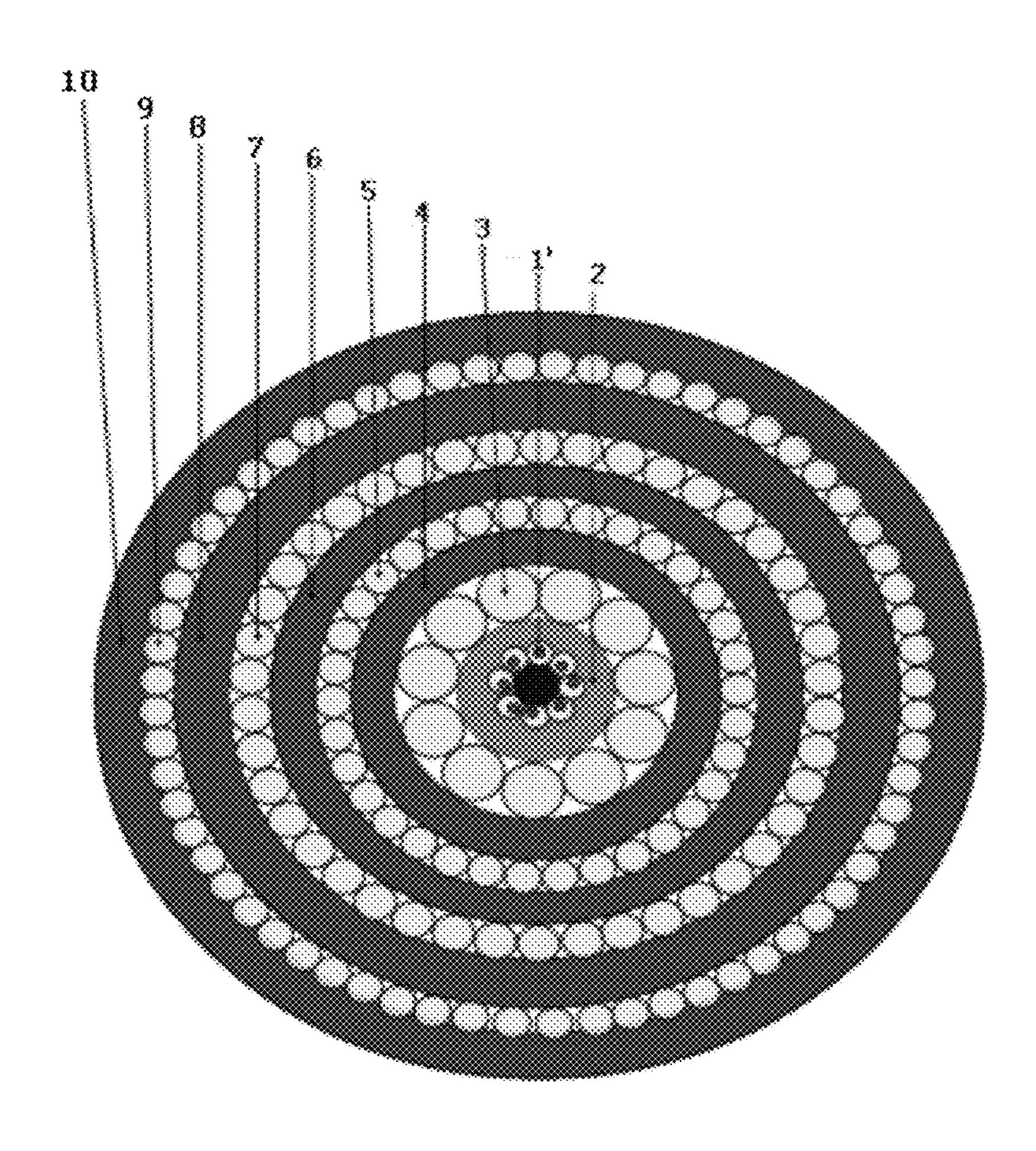
OVERHEAD CABLE FOR THE TRANSMISSION OF LOW-VOLTAGE AND MEDIUM-VOLTAGE ELECTRIC POWER AND DIGITAL SIGNAL, ALUMINUM ALLOY CONCENTRIC CONDUCTORS WITH A FIBER-OPTIC CABLE INSIDE AND DRAWN WIRE TREATMENT PROCESS
