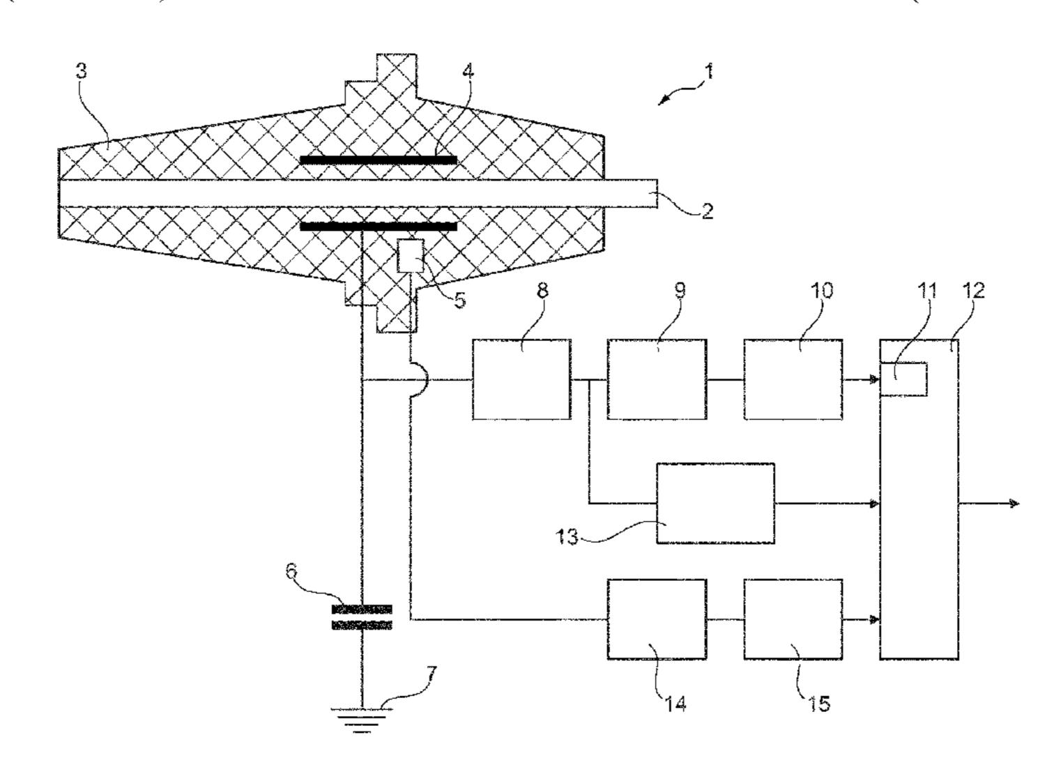
to provide a capacitive voltage divider with the first capacitor; and a voltage measurer for measuring the voltage at the capacitor plate, the voltage measurer including a frequency measurer for measuring the frequency of the voltage in the conductor and an AC voltage calculator for calculating the AC voltage in the conductor based on the capacities of the first and second capacitors, the measured voltage, and the measured frequency.
