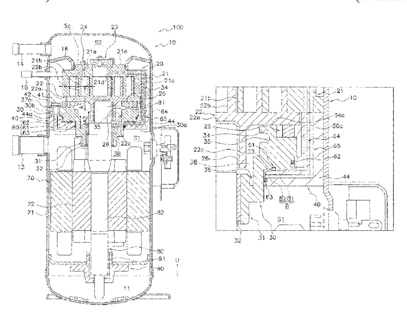
space into first and second chambers. The first flow passage guides the refrigerant in the middle of compression in the compression mechanism to the first chamber. The second guides the refrigerant discharged from the compression mechanism to the second chamber.
